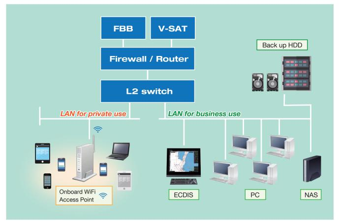
Fig. 5 Construction example of ship's LAN
